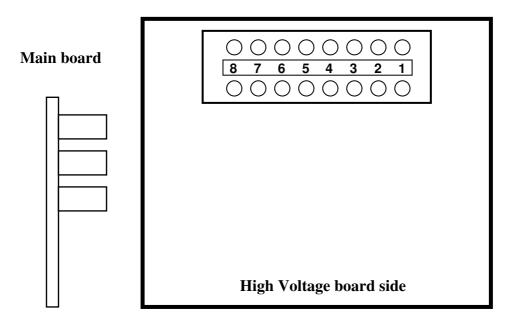
If the voltage of the power system is different from the default configuration you will have to change the position of the connector cables as shown in the table. The cables are marked from A to H and the connection points from 1 to 8.:
